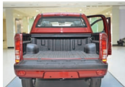
Embedded cargo compartment guard
