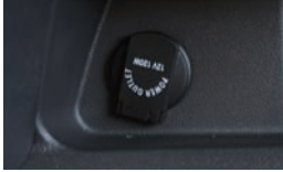
Auxiliary power socket (AC120V)
