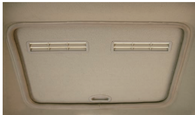
Top emergency window
