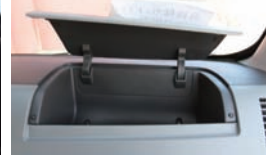
Front passenger's upper glove compartment (except models with front passenger side air bag)
