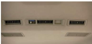
Rear A/C and integrated air outlet
