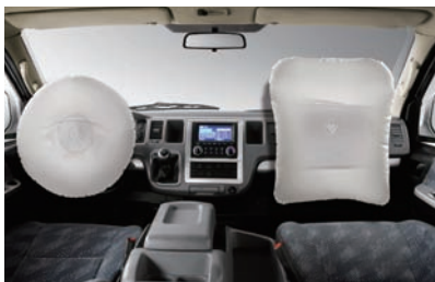
Driver/front passenger side dual air bag
