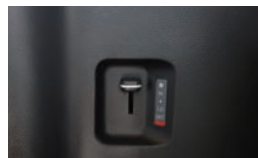
Rear air conditioner regulating switch
