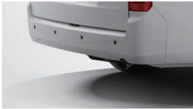
Backup sensor with 4 probes can sense the driver's blind zone effectively
