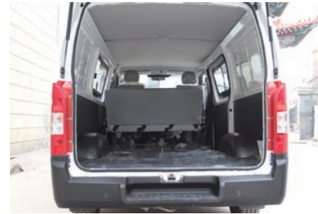
Aluminum alloy floor surfacing
