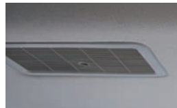
Negative ion air purifier (optional for models without optional sun roof)
