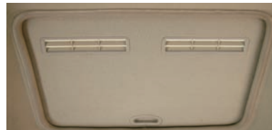
Top emergency window
