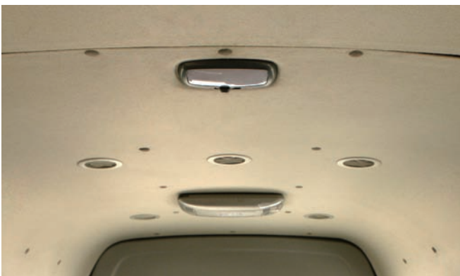
Concise roof without air outlet + semi-covered interior trims
