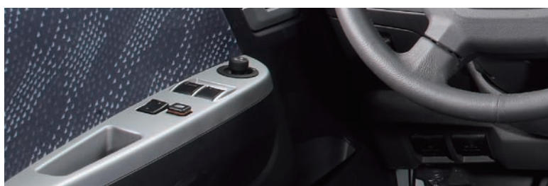
Central control door lock power window (one-touch control)
