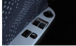
Power window (ON OFF one-touch drop on driver's seat)
