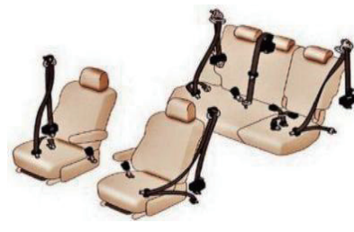
Vehicle three-point pretensioner seat belts
